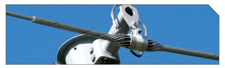
The Fiberlign Suspension provides superior cable and fibre protection at the support point. The combination of structural reinforcing rods, outer rods, 'boltless' housing and resilient inserts reduces compression, clamping, and bending stresses on cable. Negative effects of wind-induced cable motion, such as aeolian vibration, galloping, and wind sway are also minimised.
